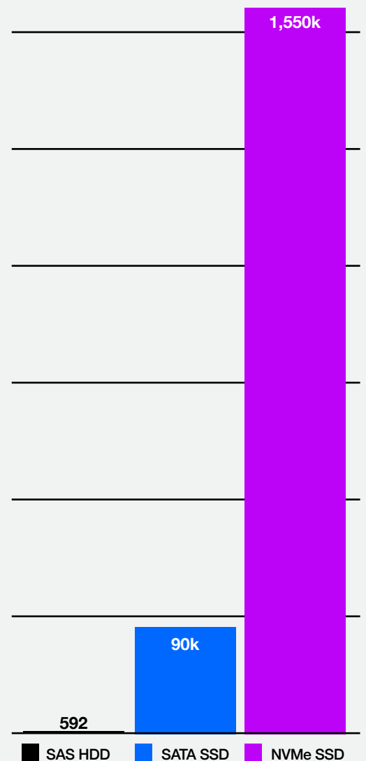
Figure 1: 4K random read IOPS for NVMe SSDs are 16x faster than SATA SSDs. 2
